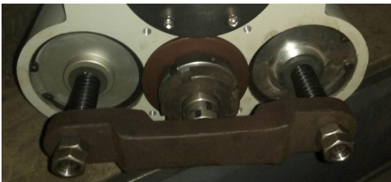
5) Two air cylinder to change the tool.
